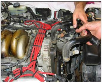
Removing Coolant Flow Tube
