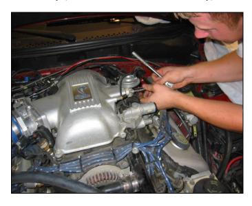
Drain down the coolant just a bit, unless you plan on replacing it. We found that siphoning out of the coolant flow tubes is the easiest way to insure you remove just enough – (To remove the intake manifold, the coolant flow tube must be loosened and removed – so you'll need to drain it down)
