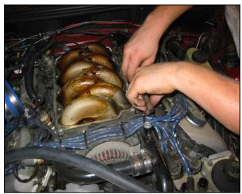
**Lifting Fuel Rails and Injectors**
