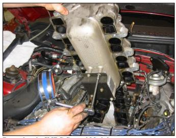
**Removing the IMRC Control Module**
